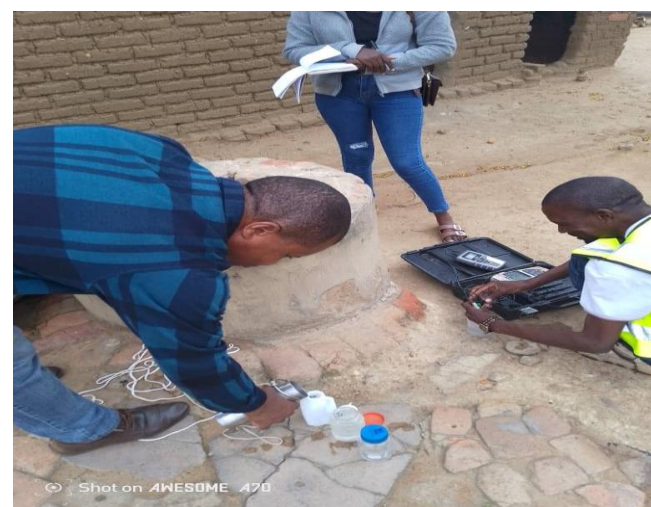
Figure 2 protected shallow well water collection
